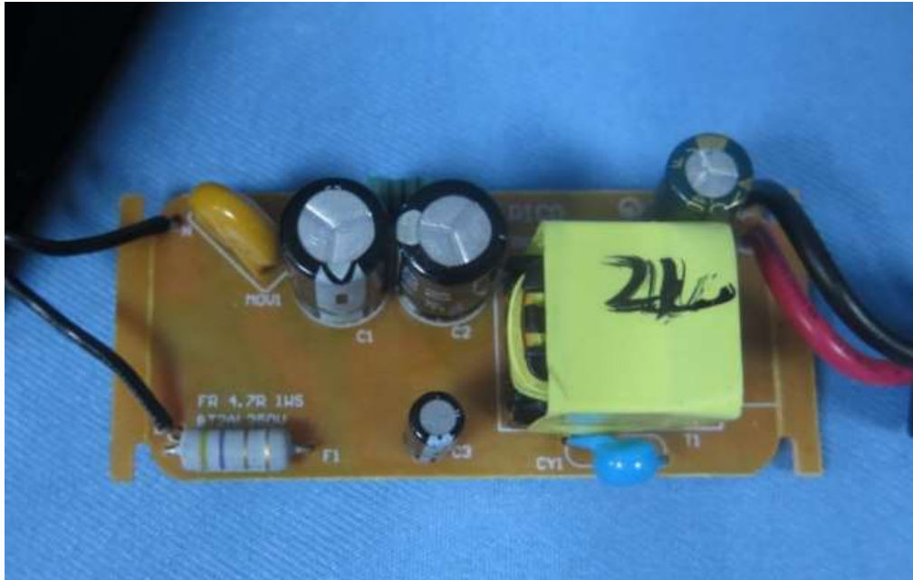
Figure 11. PCB component side view of model RKPO-zzxxxxyyy-D2 (after removed glue)
