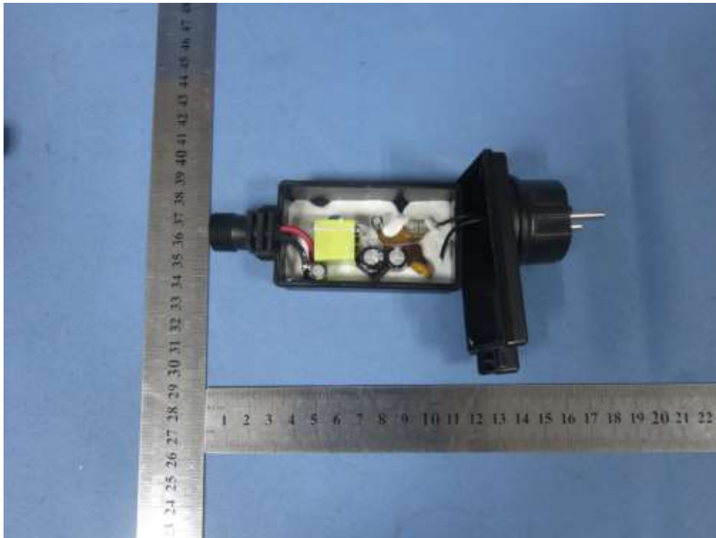
Figure 10. Internal view of model RKPO-EUxxxxyyy-D2
