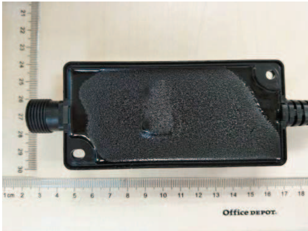
Figure 43. Internal view of RKPO-zzxxxxyyyCD-5 (with glue)
