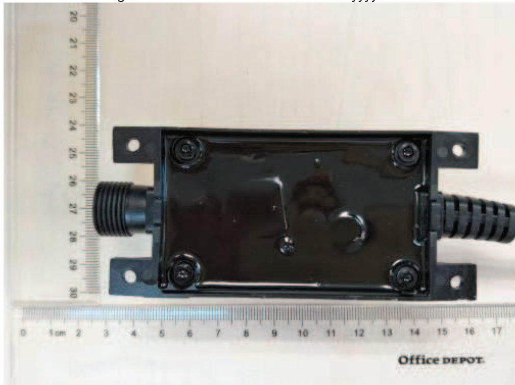
Figure 50. Internal view of RKPO-zzxxxxxyCD-2 (with glue)
