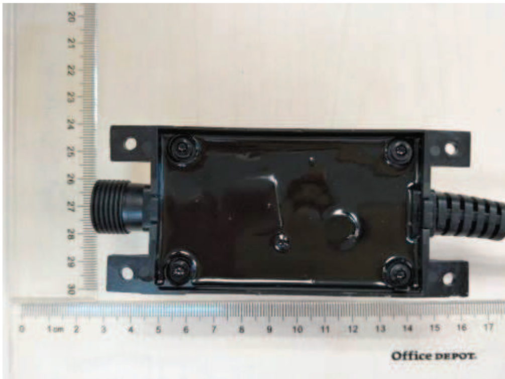
Figure 54. Internal view of RKPO-zzxxxxyyyCD-1 (with glue)
