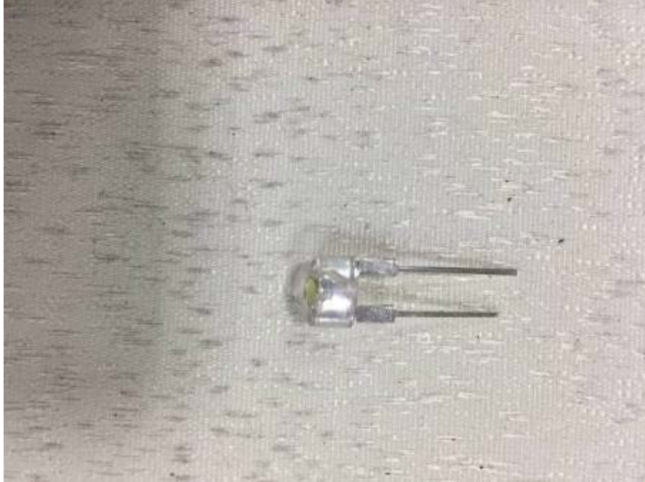
LED Source: 8MM power straw hat white super bright LED (EBO authenticate the photo on original report only)
